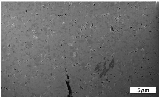
Fig. 5. A SEM micrograph of the 0.5BT-0.5KN ceramics prepared at  $T_2$  of 1095°C.
