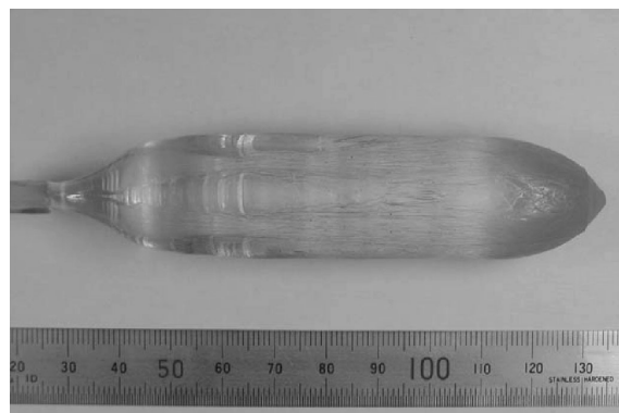
Fig. 1. As grown \text{La}_3\text{Ta}_{0.5}\text{Ga}_{5-x}\text{Al}_x\text{O}_{14} ( x = 0.3 ) single crystal.
