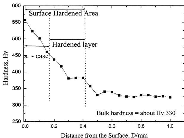
Fig. 5 Hardness distribution of Ti6Al4V alloy castings in  $ZrO_2$  mold.
