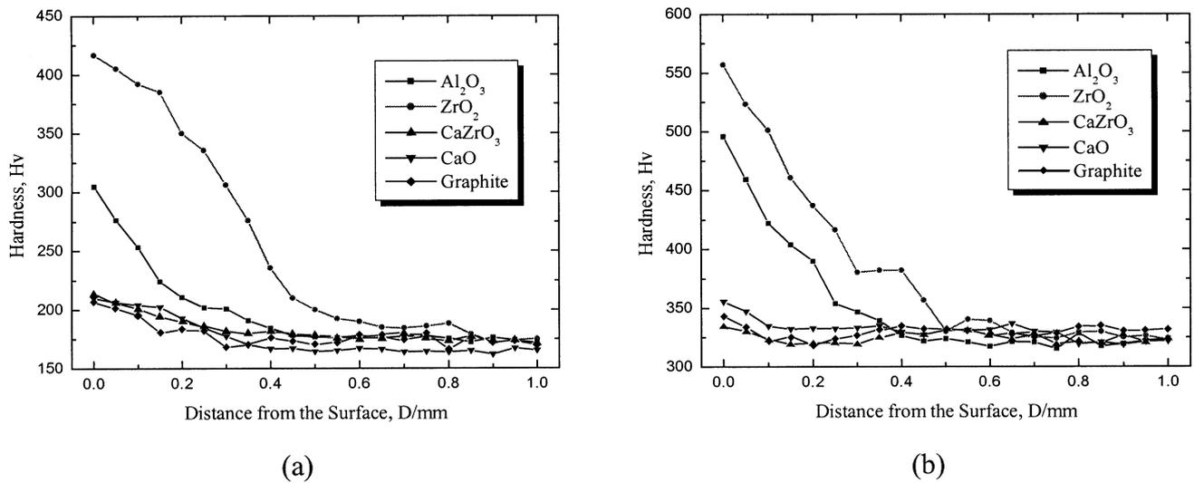
Fig. 3 Effect of mold materials on hardness profiles of (a) CP Ti and (b) Ti6Al4V alloys.
