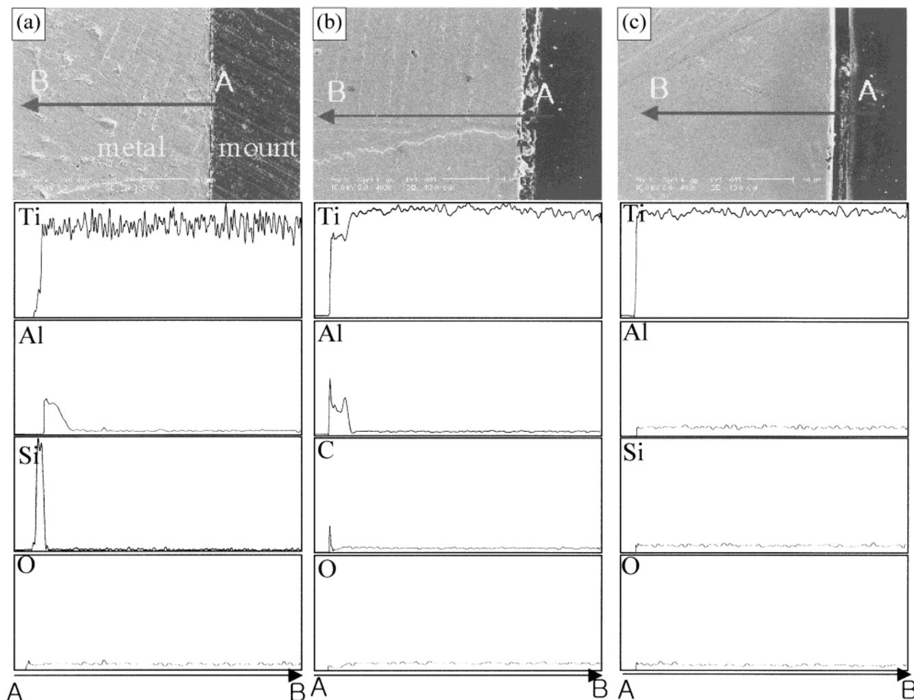
Fig. 7 Results of EDS line scanning of the regions below the surface of the castings with different binders; (a) colloidal silica, (b) acetic acid, and (c) aqueous solution.
