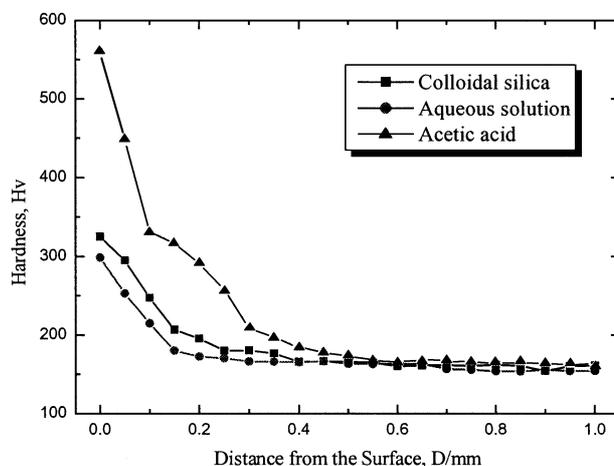
Fig. 6 Effect of the binders on microhardness profile of commercially pure titanium into  $Al_2O_3$  mold.
