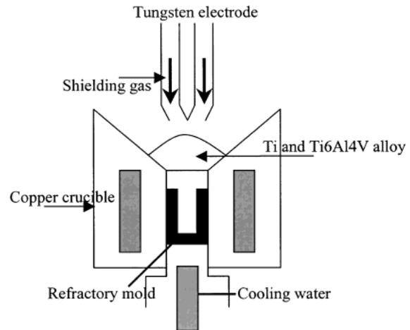
Fig. 2 Schematic diagram of plasma arc melting furnace.
