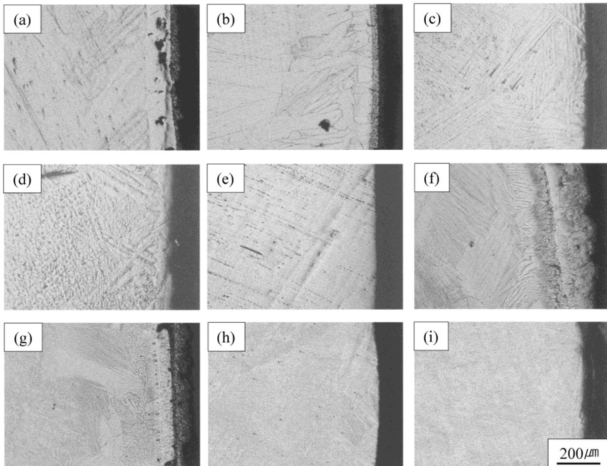
Fig. 4 Photographs showing microstructures of regions below the surface of the as-cast (a) CP Ti in  $\text{ZrO}_2$  mold, (b) CP Ti in  $\text{Al}_2\text{O}_3$  mold, (c) CP Ti in  $\text{CaO}$  mold, (d) CP Ti in graphite mold, (e) CP Ti in  $\text{CaZrO}_3$  mold, (f) Ti6Al4V in  $\text{ZrO}_2$  mold, (g) Ti6Al4V in  $\text{Al}_2\text{O}_3$  mold, (h) Ti6Al4V in  $\text{CaO}$  mold, and (i) Ti6Al4V in  $\text{CaZrO}_3$  mold, respectively.
