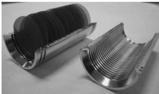
Fig. 3 Cartridge system with a lid which includes SUS meshes.
