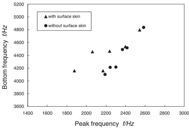
Fig. 6 Relationship between frequencies at bottom (minimum) and peak (maximum) absorption coefficient.
