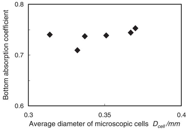
Fig. 12 Relationships between bottom absorption coefficients and urethane foam cell diameter.
