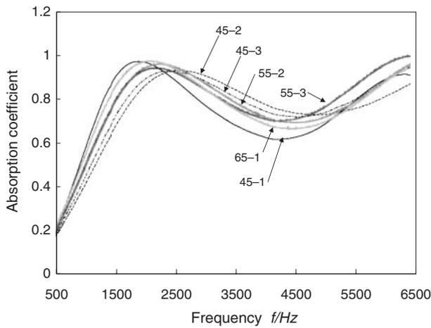
Fig. 2 Measured normal incidence acoustic absorption coefficient for samples with surface skin.
