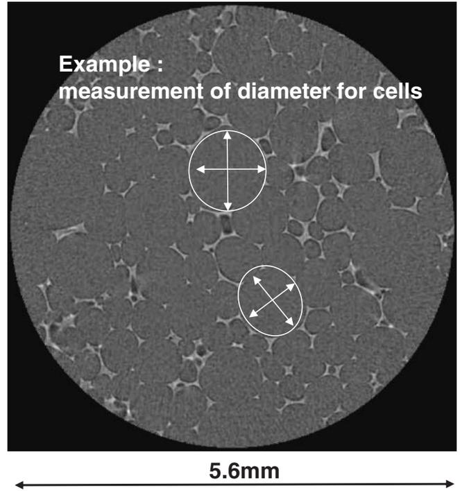
Fig. 10 Definition of evaluation value for cell structure of urethane foam based on X-ray CT photograph.
