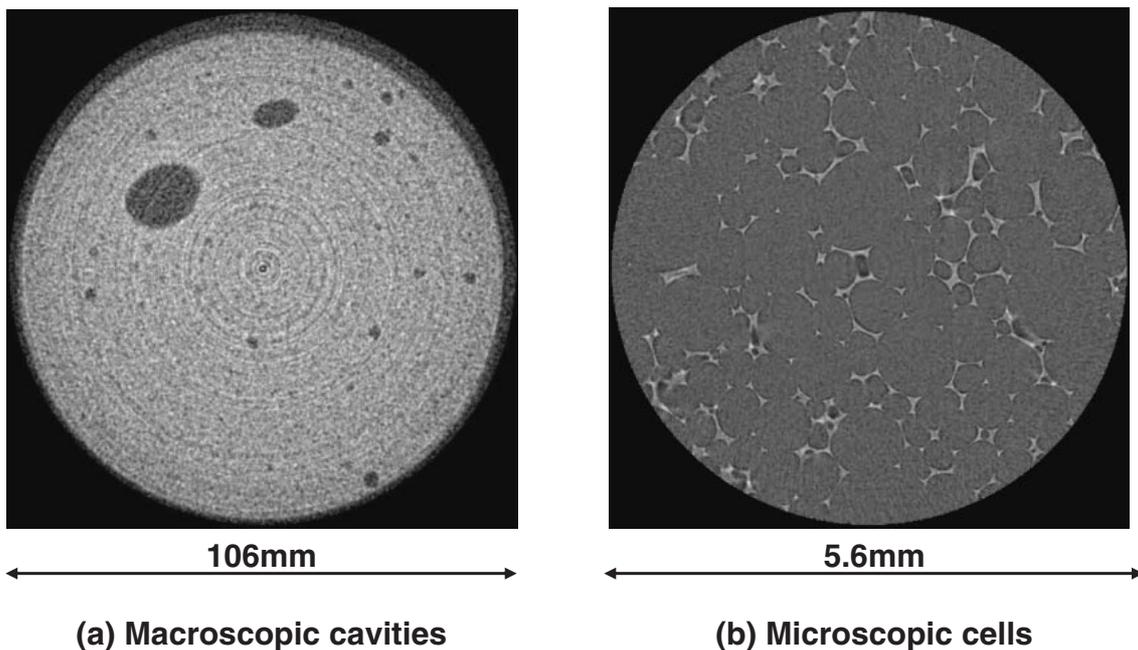
Fig. 7 Two observed cross sections by X-ray CT.
