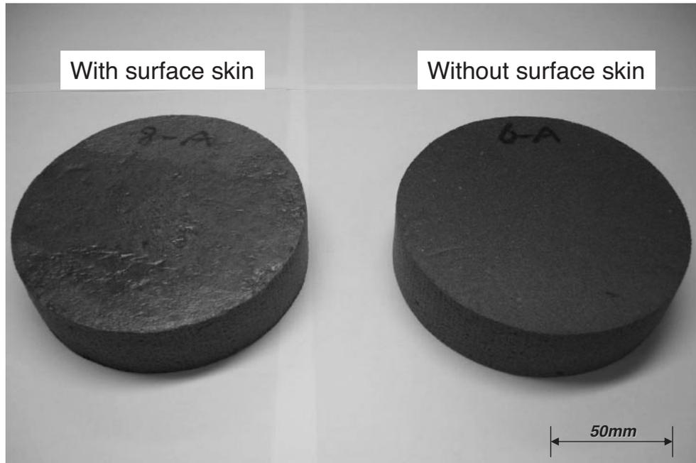
Fig. 1 External appearance of samples: a thin skin is evident on the lower temperature sample (left) but not on the higher temperature sample (right).
