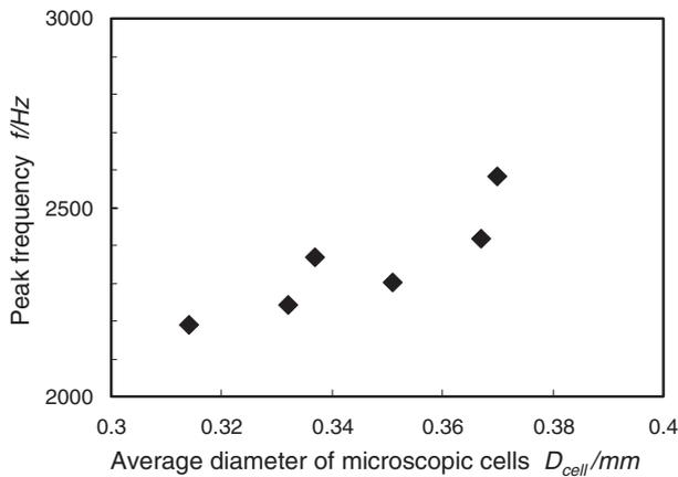
Fig. 13 Relationships between peak frequencies and urethane foam cell diameter.
