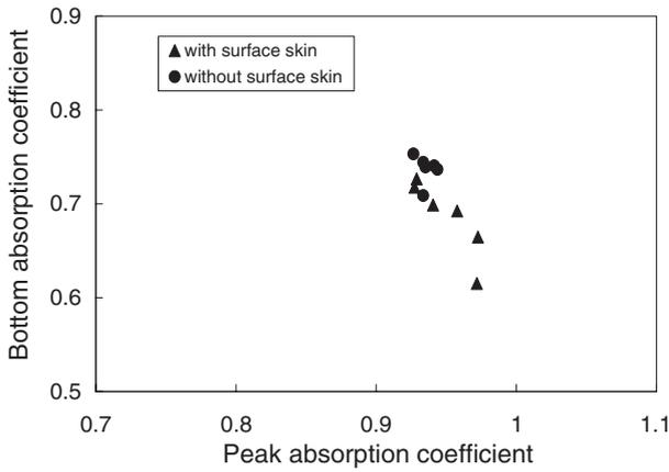
Fig. 5 Relationship between absorption coefficients of bottom (minimum) and peak (maximum).
