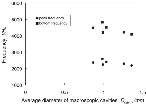
Fig. 9 Relationship between frequency and average diameter of macroscopic cavity.
