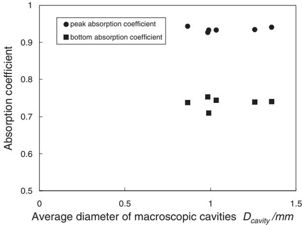
Fig. 8 Relationship between absorption coefficient and average diameter of macroscopic cavities.
