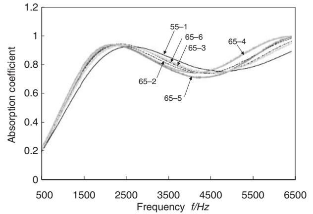
Fig. 3 Measured normal incidence acoustic absorption coefficient for samples without surface skin.
