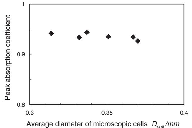
Fig. 11 Relationships between peak and bottom absorption coefficients and urethane foam cell diameter.
