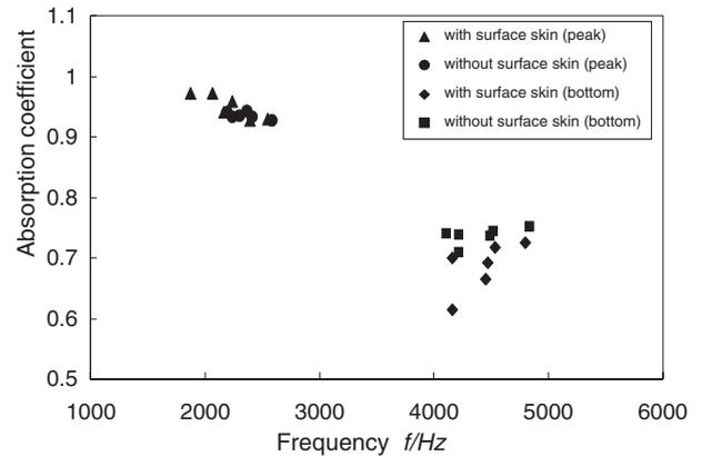
Fig. 4 Relationships between peak absorption coefficient and peak frequency and between bottom absorption coefficient and bottom frequency for samples with and without surface skin.
