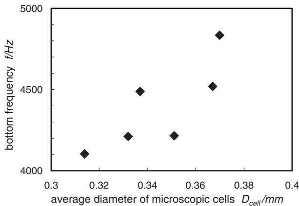
Fig. 14 Relationships between bottom frequencies and urethane foam cell diameter.
